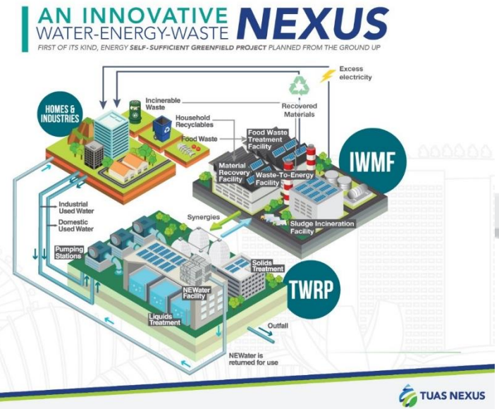
Infographic on Tuas Nexus. Photo credit: The National Environment Agency (NEA) and PUB, Singapore’s National Water Agency
