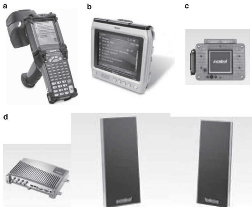
Figure 4 RFID equipment: (a) handheld RFID readers; (b) mobile computer; (c) RFID reader for forklift; (d) Gantry reader and antenna.
